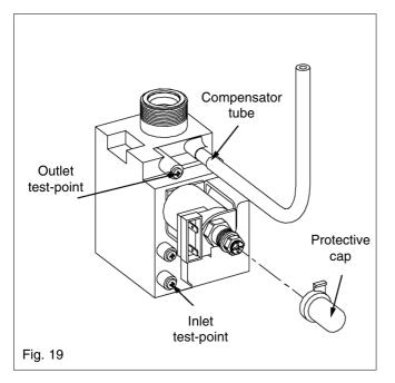
Once the burner pressure has been checked, close the DHW outlet, isolate the appliance from the electrical supply, remove the manometer, and tighten the gas valve outlet test nipple.
