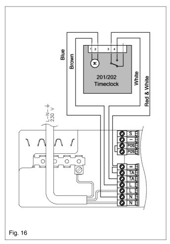
Connect the supply cable wires (LIVE, and NEU-TRAL) to their corresponding terminals on the appliance terminal block. Connect the EARTH wire to the EARTH block (see fig. 16) ensuring that it's left slightly longer that the others, this will prevent strain on the EARTH wire should the cable become taut.
