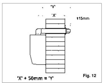
Seal the flue assembly to the wall using cement or a suitable alternative that will provide satisfactory weatherproofing. The interior and exterior trim can now be fitted.
