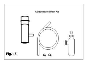
The condensate drain kit must be fitted within 1 metre of the appliance flue outlet. It is recommended that the condensate drain kit should be fitted in the vertical plane, however it can be fitted horizontally with care.
