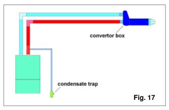
A 130mm hole is required for the passage of the concentric terminal through the wall.
