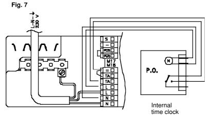
Fig. 7 Showing 230v input electrical connection and internal timer without room thermostat.
