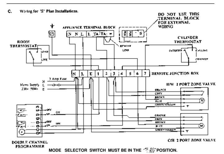
To ease wiring conjection at the appliance terminal strip, remove the wiring harness normally used for internal clock connection.
