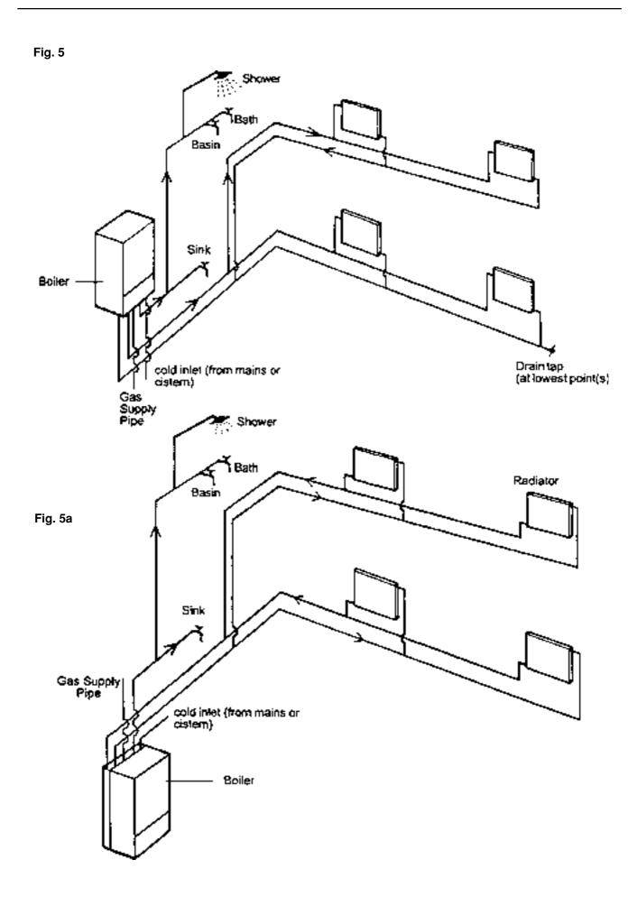
**N.B.** Vokèra Ltd recommend a 2-pipe system. Single pipe systems are more liable to be troublesome unless carefullly designed and installed.
