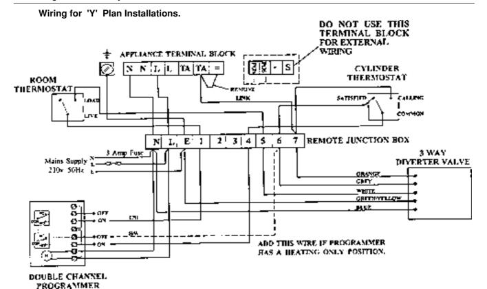
NOTE: WHEN USING A 'Y' PLAN INSTALLATION THE MODE SELECTOR SWITCH WILL BE OVERRIDEN BY THE CONTROL CIRCUIT.
