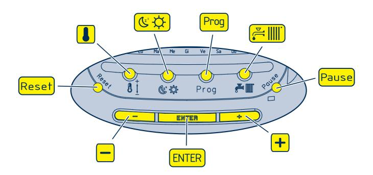
Regulates the heating and domestic hot water temperature
