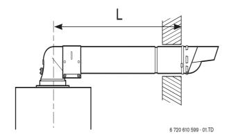
Fig. 23 Flue length - side
