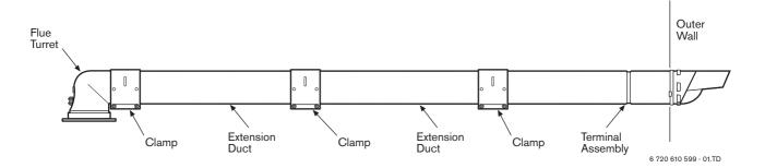
Fig. 20 Flue with extensions
