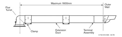
Fig. 19 Flue with one extension
