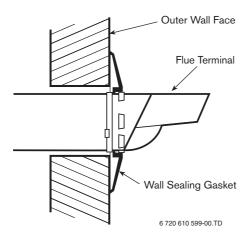
Fig. 24 Flue terminal position
