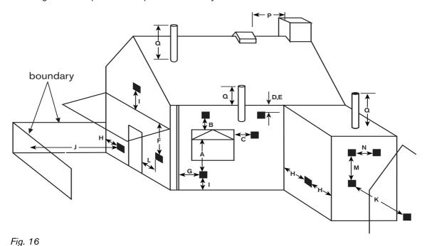
Minimum dimensions of flue terminal positions (all types) (see fig. 16)
