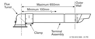
Fig. 18 Standard Flue
