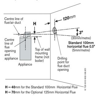
Fig. 17 Marking the position of the side flue opening. Note: ensure there is adequate access to the air/flue sampling points in the flue turret.
