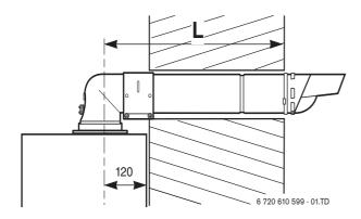
Fig. 22 Flue length - rear
