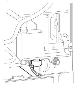
Fig. 13 Recommended route of the condensate drain
